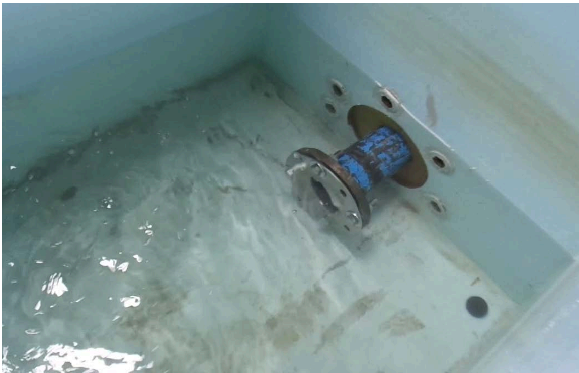
Figure 2. Test Setup for the Submerged 4-Inch Rubber Check Valve Tests
