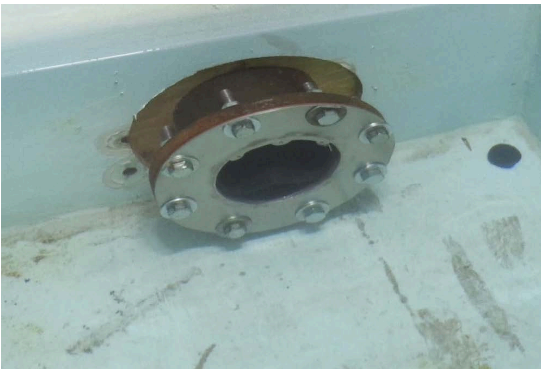
Figure 2. Test Setup for the Submerged 8-Inch Rubber Check Valve Tests
