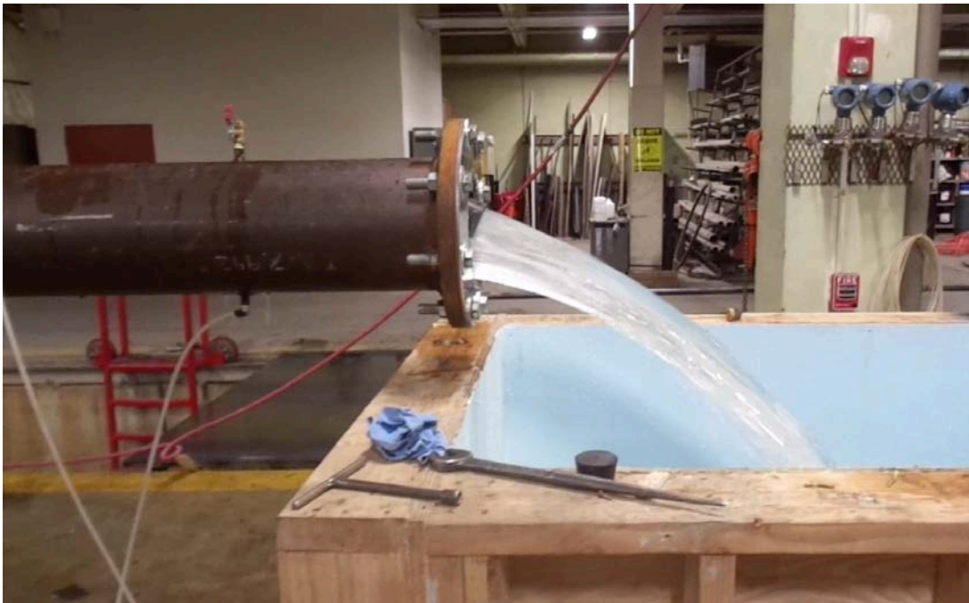
Figure 1. Test Setup for the Free-Discharge 8-Inch Rubber Check Valve Tests
